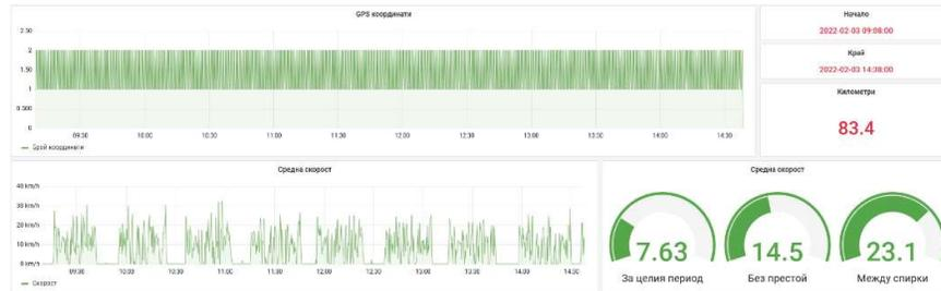
**Fig. 4.** Example technical output, showing distance travelled, GPS coordinate quality and average speed between different stops.
